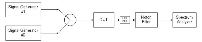
Figure 1 - Reverse Path Intermodulation Test Setup
