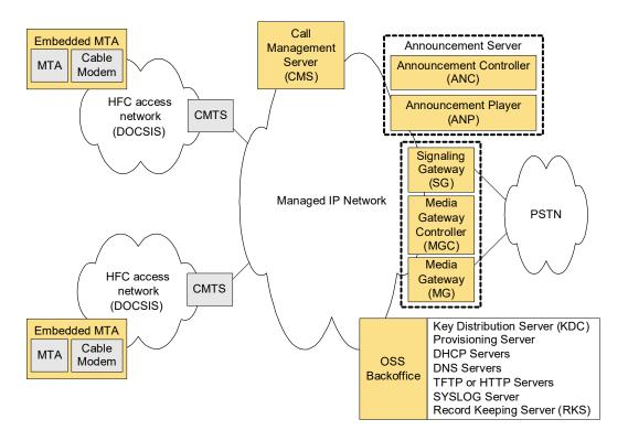
Figure 1. IPCablecom Network Component Reference Model
