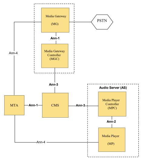
Figure 2. IPCablecom Audio Server Components and Interfaces
