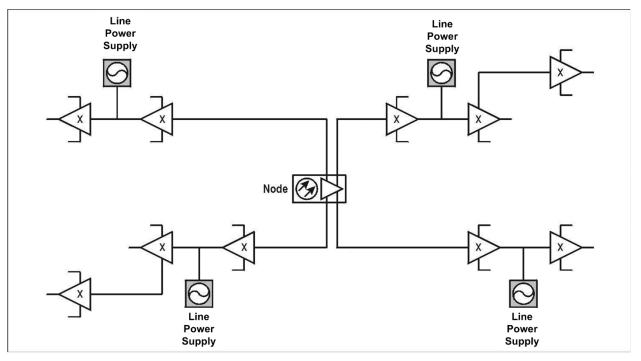
Figure 1 - Typical HFC Powering
