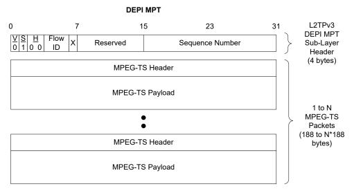
Figure 8–3 - DOCSIS MPT Sub-layer Header and Payload
