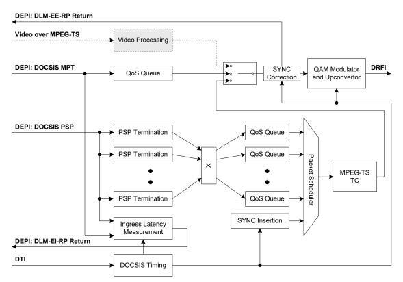
Figure 6–1 - Downstream EQAM Block Diagram
