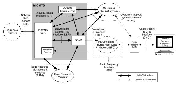
Figure 5–1 - Modular CMTS Reference Architecture
