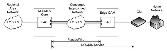
Figure 7–1 - L2TP Topology for Modular CMTS
