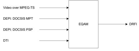
Figure 5–2 - EQAM Block Diagram
