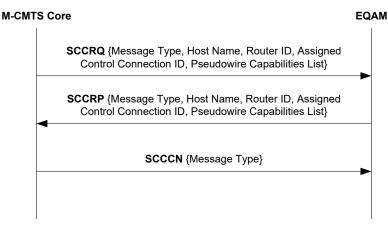
Figure 7–6 - DEPI Control Connection Setup
