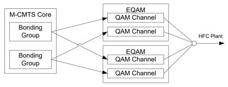
Figure 5–3 - Bonding Services Model
