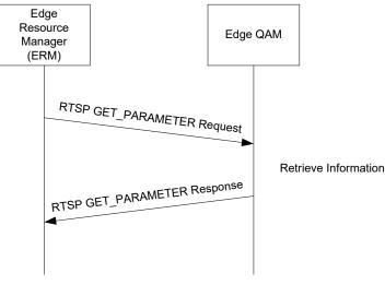
Figure 7–3 - GET\_PARAMETER Interaction Diagram
