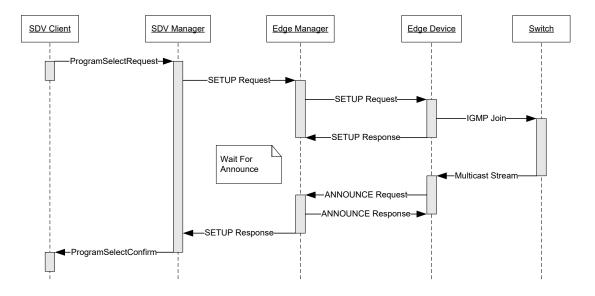
Figure I–3 - Message Flow for Synchronous Mode
