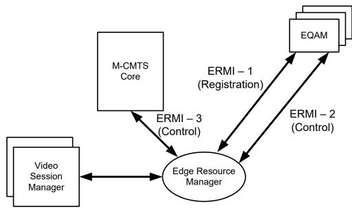
Figure I–1 - Use Case, base architecture
