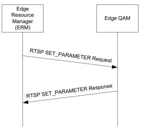
Figure 7–2 - Keepalive Interaction Diagram
