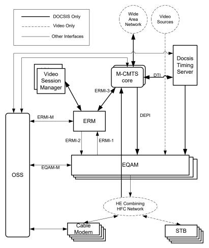
Figure 1–1 - M-CMTS Reference Architecture
