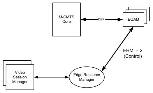
Figure 5-4 - Simplified Framework for Static QAM Partitioning
