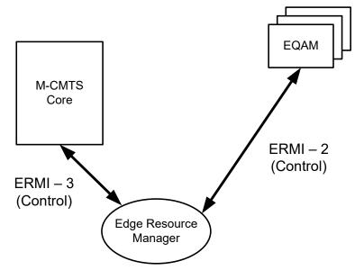
Figure 5-3 - Resource Allocation Interfaces and Components
