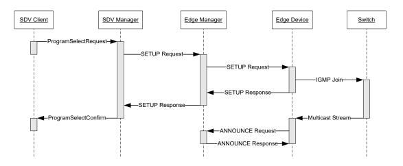
Figure I-4 - Message Flow for Asynchronous Mode
