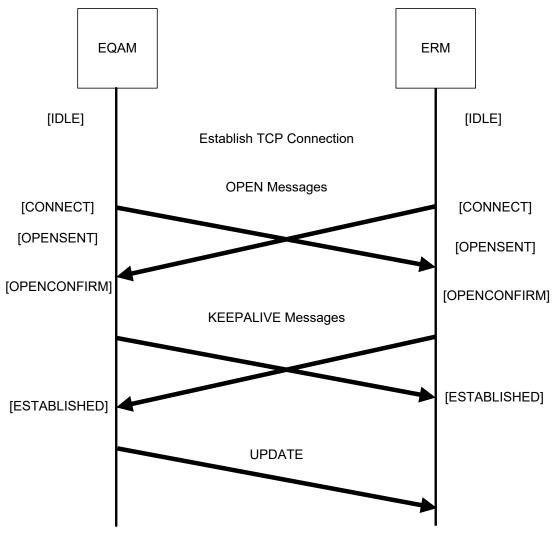
Figure 6–29 - Example ERRP Connection Establishment
