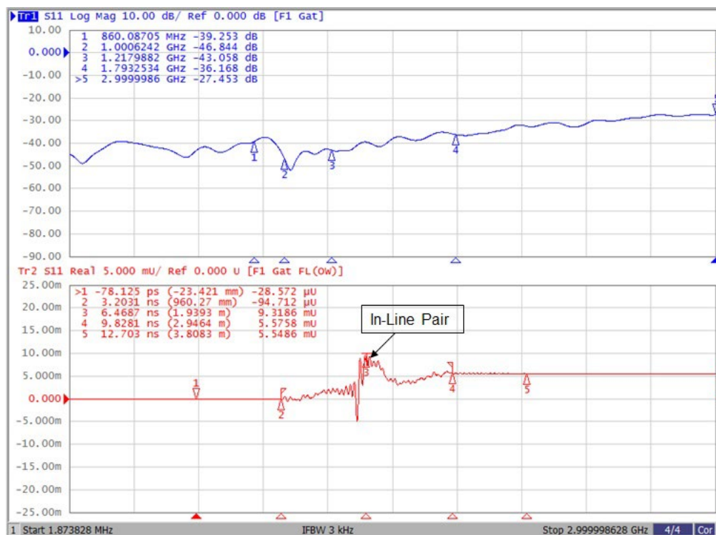
Figure 3 - Time Gated Response of In-Line "F" Connector Pair
