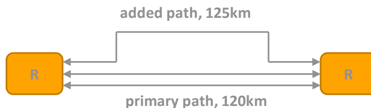
Figure 8 - Physical path asymmetry in a LAG bundle
