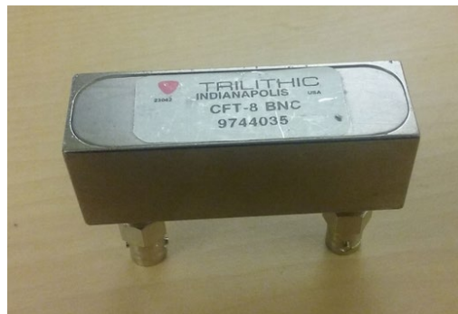
Figure 3 – A bandpass filter used for lab tests.
