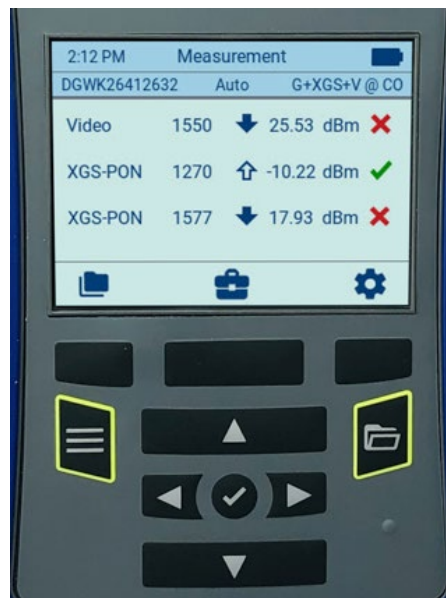
Figure 6 - PON power meter evaluates pass/fail of detected PON power levels.
