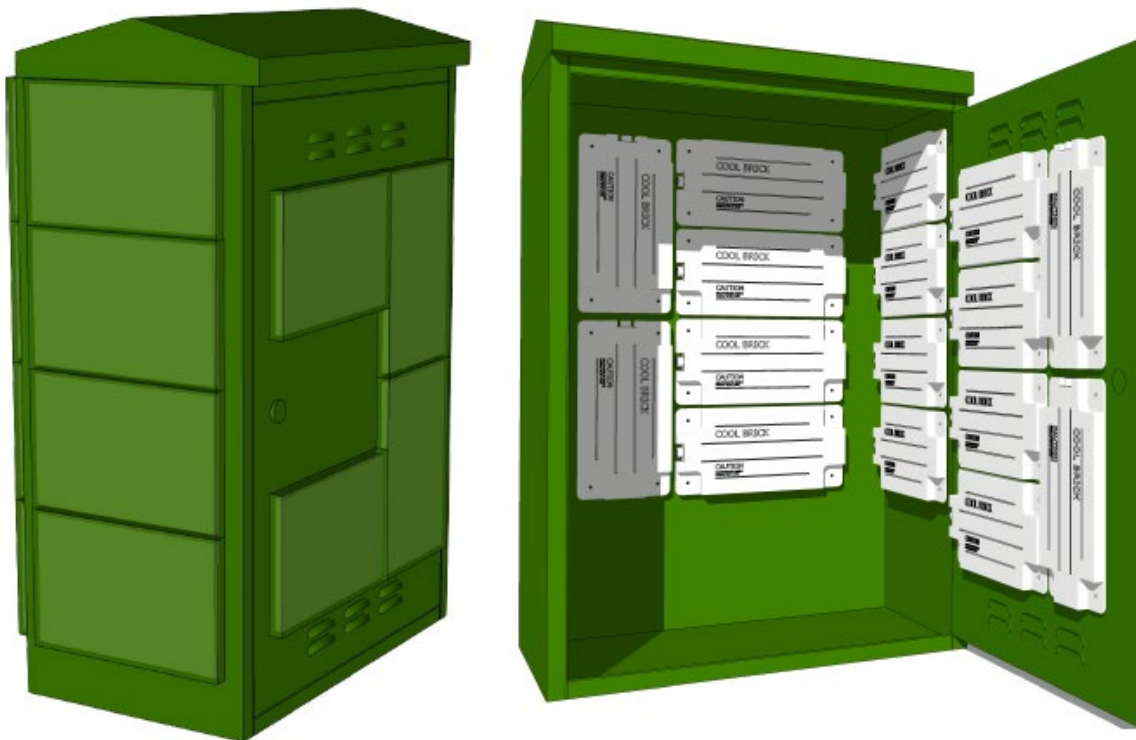
Figure 3 -Passive Cabinet Cooling Installtion Example
