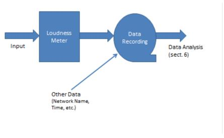
Figure 1: High-level measurement equipment configuration
