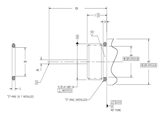
Figure 1 - Physical Dimensions for 5/8-24 Plug, (Male), Trunk & Distribution Connectors
