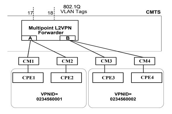
Figure I-2 - Multipoint L2VPN Forwarding of Traffic Example
