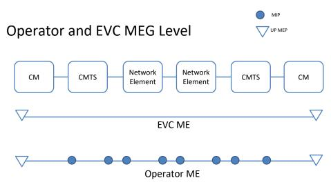
Figure 8-1 - Operator and EVC MEG Level
