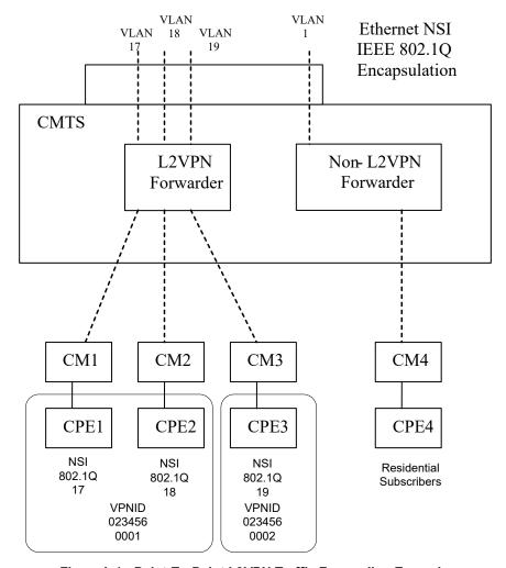
Figure I–1 - Point-To-Point L2VPN Traffic Forwarding Example
