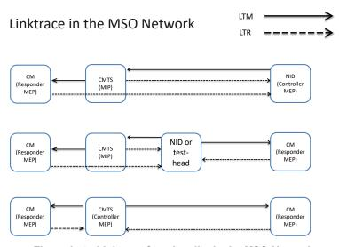
Figure 8-4 - Linktrace functionality in the MSO Network
