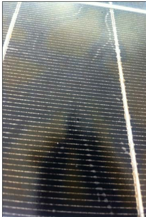
Figure 11 - Cracks in Cells Caused By Flexure of the Panel at the Factory
